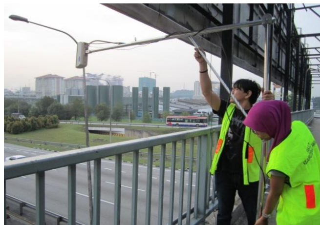
Fig. 1: Specially fabricated tripod for CCD camera.
